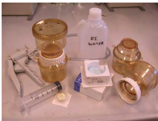
Figure 1.8. Filtration equipment for water sampling, showing (L to R) hand pump, syringe and small filter, Nalgene® filter unit, filter papers, deionised water and another filter unit.
