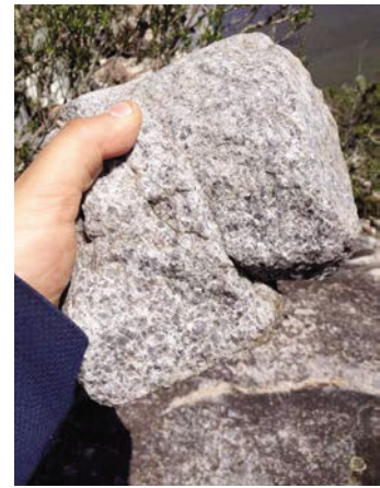
Figure 18. Well-sorted, pebble conglomerate quartzite, Mount Ragged (MGA 543627E, 6297322N); Sample MRF_03 (Figure 13i & j).
