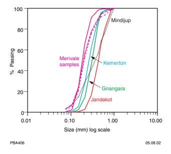
Figure 54. Particle-size distribution of sand from Merivale area and operating silica sand mines in Western Australia
