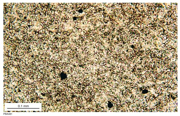
Figure 84. a) Photomicrograph (ordinary light ×20) showing contorted to undulating extremely fine layering of chlorite in chert (sample GSWA145228: Moora silica mine); b) Photomicrograph detail from Figure 84a showing ultrafine chlorite crystals and opaque minerals (ordinary light ×200)
