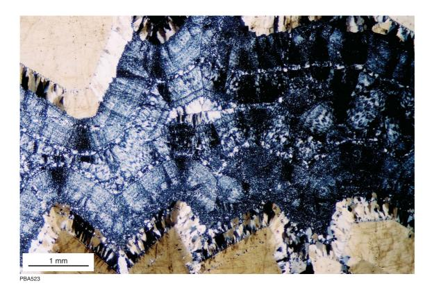
Figure 135. Photomicrograph (crossed nicols) showing composite coarse band with coarse sparry/pyramidal quartz crystals lining the margins, with a central core of zoned chalcedonic silica (sample GSWA145210: 23 km southeast of Shaw River)
