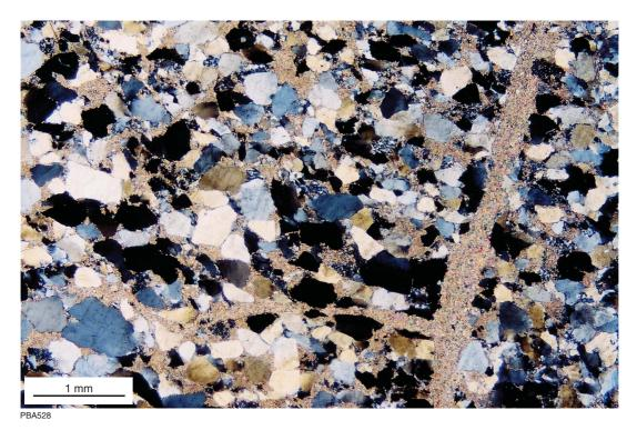
Figure 141. Photomicrograph (crossed nicols ×20) showing sericite veinlets crosscutting quartzite (sample GSWA145212: Whim Creek)
