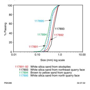
Figure 19. Particle-size distribution of silica sand — Jandakot (117891–95 are GSWA samples nos)
