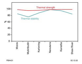
Figure 98. Average thermal stability and thermal strength of silica rocks from various localities of Western Australia
