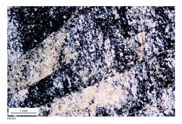
Figure 148. Photomicrograph (crossed nicols ×20) showing large-scale breccia domains, with angular, sharpblocky outlines, and straight fracture traces (sample GSWA145224, Location E, Fig. 142)
