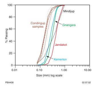
Figure 56. Particle-size distribution of sand from the Condingup area and operating silica sand mines in Western Australia
