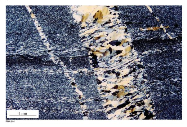
Figure 129. Photomicrograph (crossed nicols ×20) showing stringers and veins (width 0.5–1.5 mm) of quartz crosscutting chert layering at a fairly high angle (sample GSWA145206: 23 km southeast of Shaw River)
