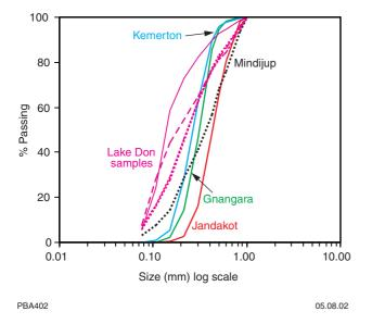
Figure 50. Particle-size distribution of silica sand from Lake Don and operating silica sand mines in Western Australia
