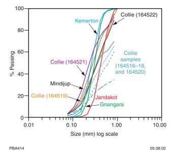
Figure 63. Particle-size distribution of sand from Collie area and operating silica sand mines of Western Australia
