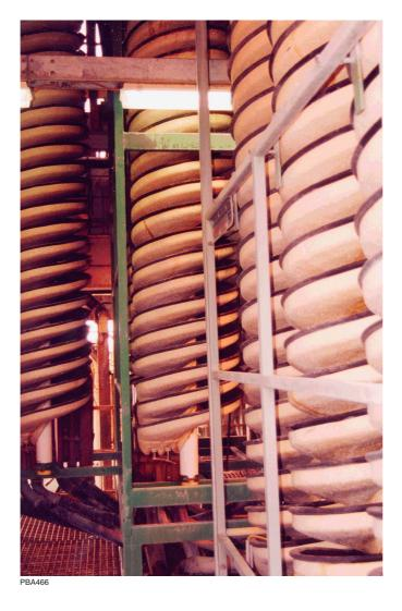
Figure 26. Spiral classifier for separating heavy minerals at Kemerton silica sand mine
