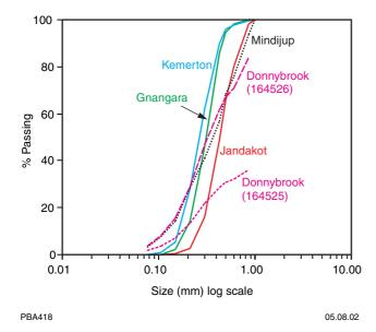
Figure 68. Particle-size distribution of sand from Donnybrook area and operating sand mines in Western Australia
