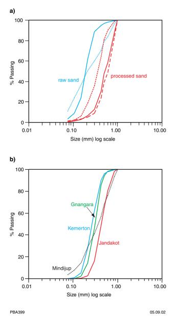
Figure 42 a) Particle-size distribution of silica sand from Mindijup mine; b) Particle-size distribution of silica sand from Mindijup mine and other operating silica sand mines of Western Australia
