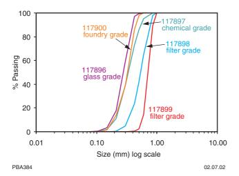
Figure 12. Particle-size distribution of silica sand — Gnangara (117896–900 are GSWA sample nos)
