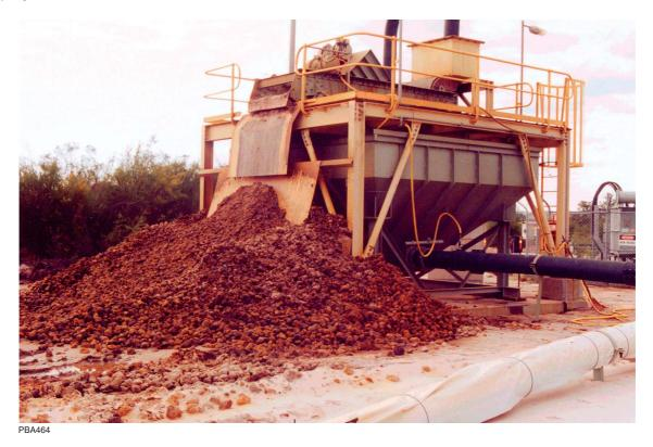
Figure 24. Washing plant for removing clay and organic material from the dredged silica sand at Kemerton silica sand mine
