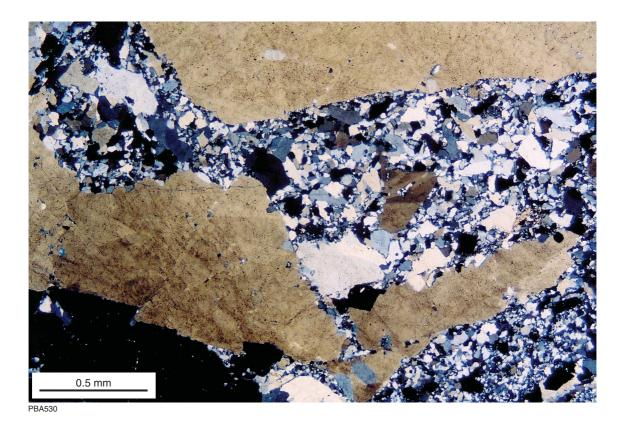
Figure 145. Photomicrograph (crossed nicols ×50) showing coarse early quartz (dusted by fluid inclusions) and a later generation of microgranular/microsparry quartz in the matrix (sample GSWA145217, Location A, Fig. 142)
