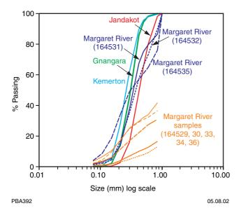
Figure 34. Particle-size distribution of sand from Margaret River region and some operating silica sand mines in Western Australia
