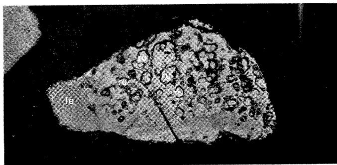
Figure 4. Photomicrographs showing alteration of ilmenite to rutile by supergene enrichment. A. Ilmenite (il) and leucoxene (le). B. Leucoxene (le) forming from amorphous iron-titanium oxide (fto). C. Rutile (ru) crystallites forming from leucoxene (le).
