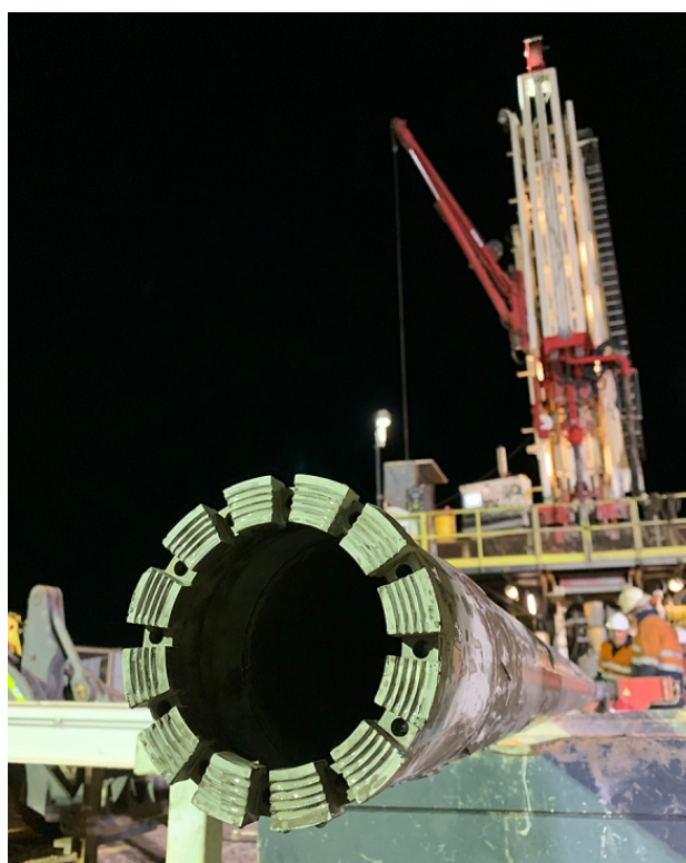
Figure 3. Fresh HQ size diamond drill bit with DDH1 Drilling's ER01 rig in the background
