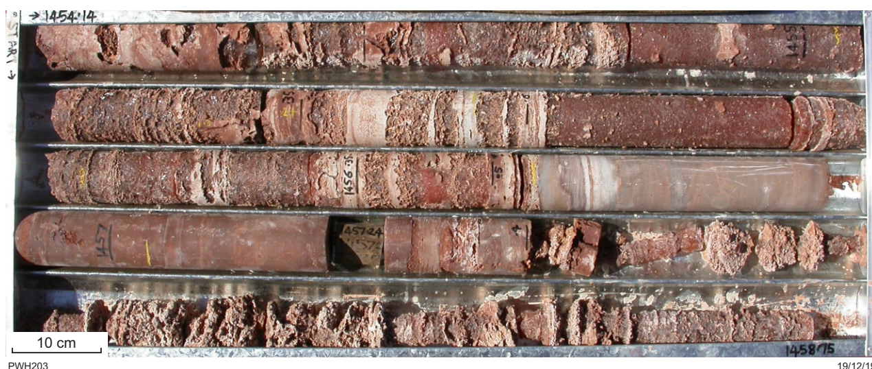
Figure 3. Interbedded halite (orange-brown) and dolomite (pale grey to grey-brown) in the lower Browne Formation in GSWA Lancer 1 (1454.14 – 1458.75 m). Significant halite dissolution during drilling is indicated near the bottom of the core tray
