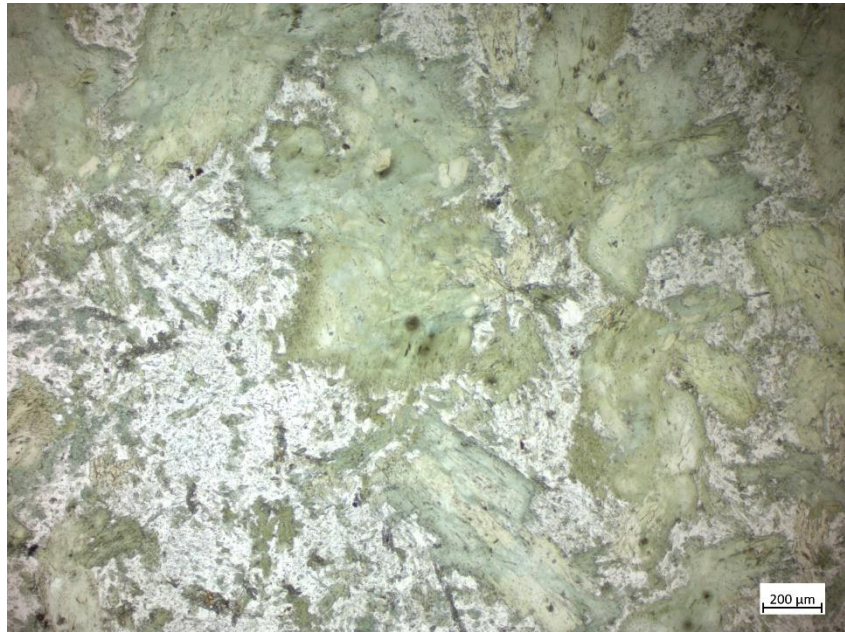
Figure 4.8: Typical texture in the Warriedar area, with amphibole pseudomorphs of coarse primary pyroxenes (green) and a feldspathic groundmass (white). Sample WR5 is pictured in plane polarized light.
