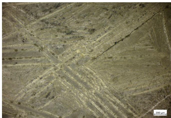
Figure 4.13: Fine bladed spinifex in sample YL8 (plane polarized light).
