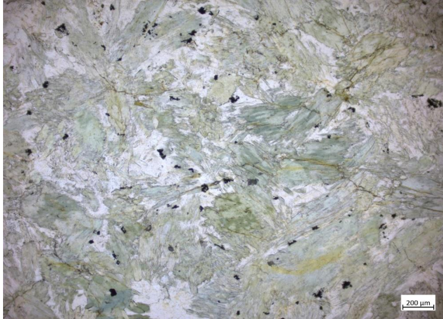
Figure 4.3: Pseudomorphs of cruciform to irregular polysynthetic twins of primary pyroxene replaced by subhedral amphibole in a fine-grained quartz-feldspar groundmass in sample MG11 (plane polarized light). The cross-type twins are typical of clinoenstatite in boninites (see text).
