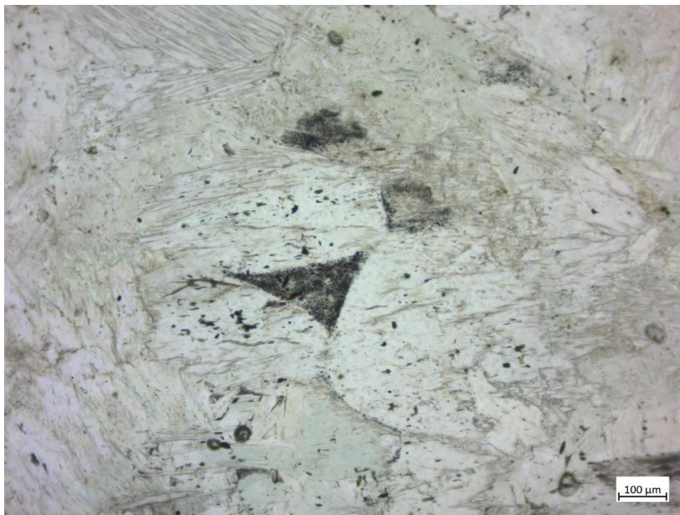
Figure 4.14: Filling in of spaces in a triangular shape in sample 225152 (plane polarized light).
