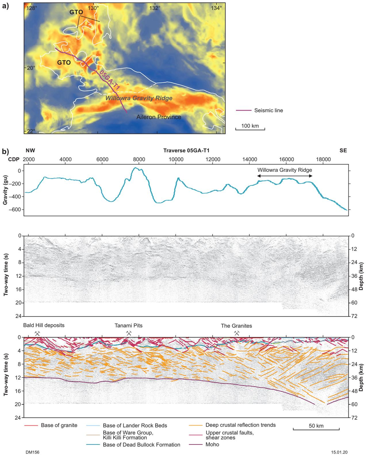
**Figure 3. Seismic reflection profile across the Granites–Tanami Orogen (GTO) and Aileron Province: a) location of seismic line on gravity image; b) raw and interpreted migrated seismic section, with gravity data collected along traverse shown at top, simplified from Goleby et al. (2009).  $V/H = 1$  at  $6 \text{ km s}^{-1}$ . Abbreviation: CDP, common depth point**
