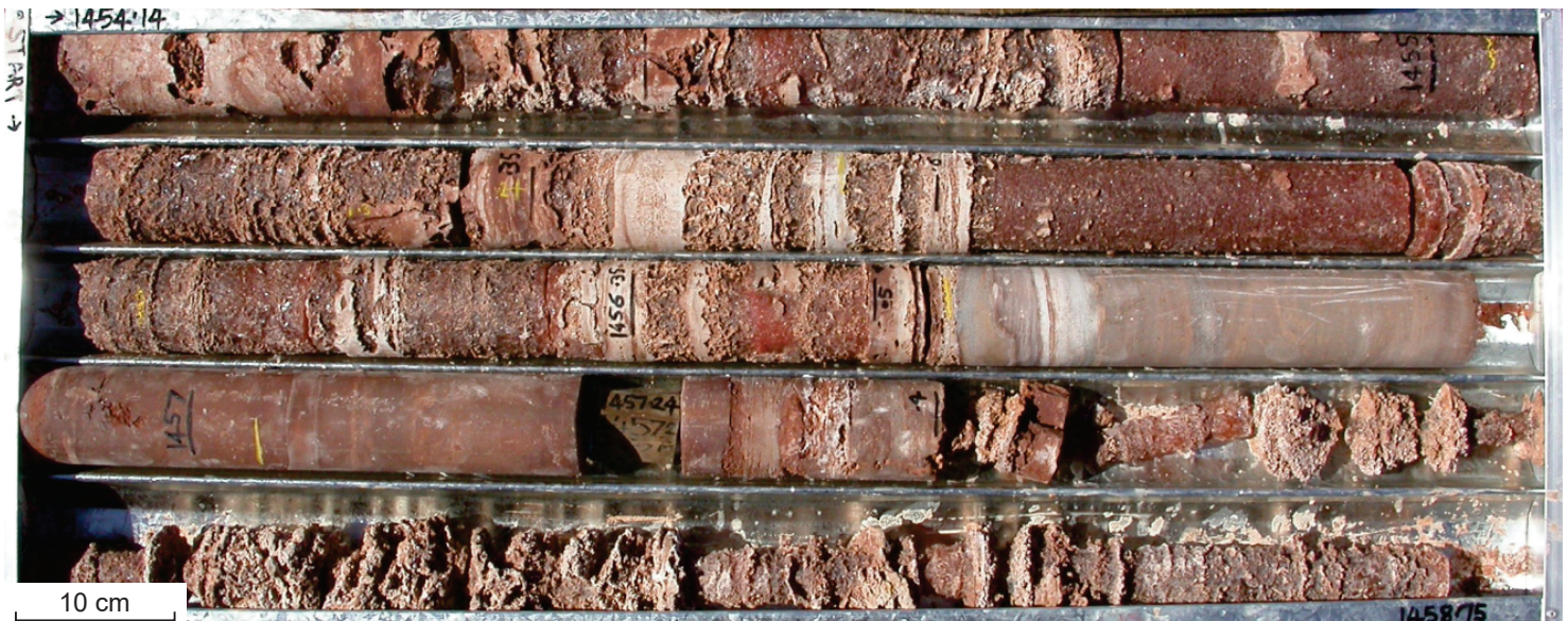
Interbedded salt and dolomite in core of the Brown Formation in stratigraphic drillhole GSWA Lancer 1
