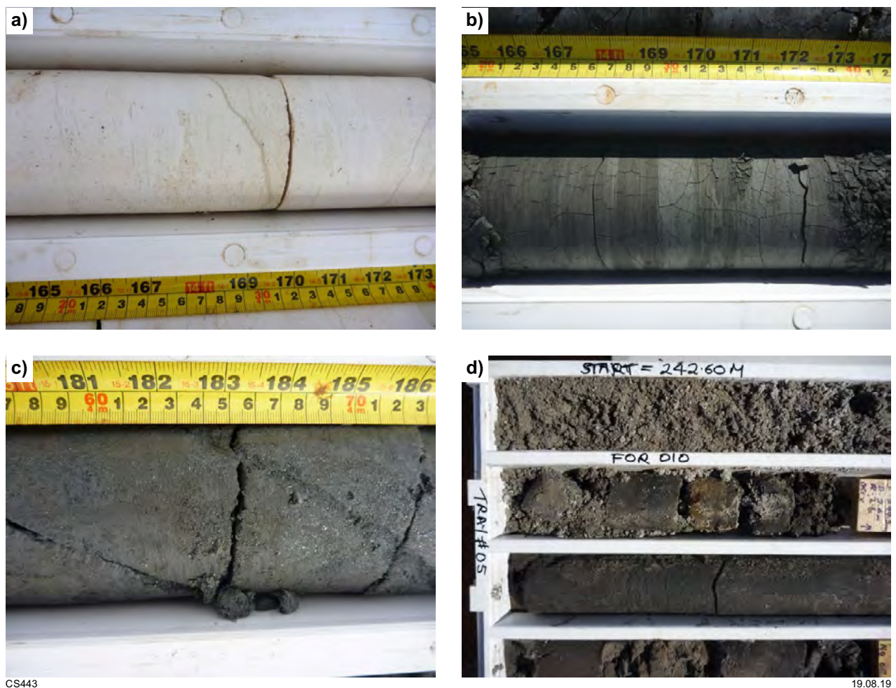
Figure 12. Photos of drillcores from the cover rocks (PQ core width 85 mm): a) typical example of Wilson Bluff limestone, drillcore FOR004; b) typical dark carbonaceous shale of the Madura Formation, drillcore FOR004; c) typical micaceous siltstone of the Madura Formation, drillcore FOR004; d) unconsolidated sand interlayered with dark siltstone, Loongana Formation, drillcore FOR010
